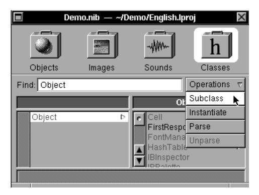
Here we define a *displayOut* outlet and a *start:* action method for the new MyObject class.
